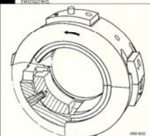
Δ Fig. 23 Four-tilting-pad radial bearing, type R 4K, for high speeds and normally used in barrel compressors.
